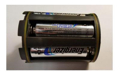
**Warning!** Do not mix battery types! Damage to the camera can result and your warranty will be voided if you mix battery types.
