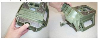
To replace the camera's cover, insert the cover along the bottom edge of the camera's faceplate and rotate it downward until it's flush with the camera. Snap the clasp, pressing firmly in the middle of the clasp, to secure the cover.
