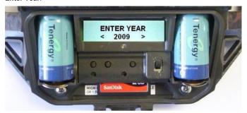
Press the << and >> buttons to set the date (year, month, and day) and time (hour and minute); press the **OK** button after each part of the date and time are correct.
