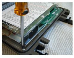
2. With power off, remove the six screws that secure the circuit board holder to the front cover of the camera case.
