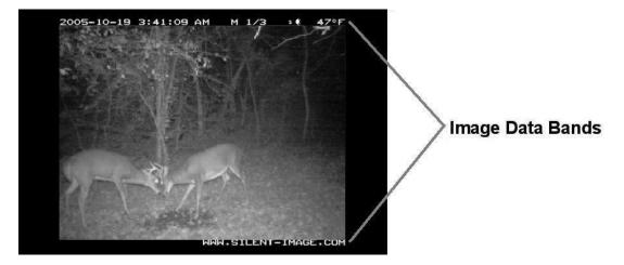
Phases of the moon displayed in the image bands include: (new moon), (waxing crescent), (first quarter), (waxing gibbous), (full moon), (waning gibbous), (last quarter), and (waning crescent). Any time the infrared illuminator is used, (the infrared illuminator "flash" indicator) appears in the Image Data bands.
