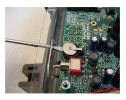
5. Slip a small, flat screwdriver under the coin battery.
