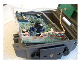
4. You can gently rest the circuit board holder on the main body of the camera case for easy access to the coin battery.
