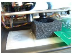
10. Place the circuit board holder in its original position on the front cover of the camera case.
