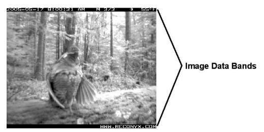
Phases of the moon displayed in the image bands include: (new moon), (waxing crescent), (first quarter), (waxing gibbous), (full moon), (waning gibbous), (last quarter), and (waning crescent). Any time the infrared illuminator is used, (the infrared illuminator "flash" indicator) appears in the Image Data bands.
