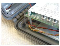
11. Be sure that the wires for power and illuminator route around the outside of the hexagonal standoff in the bottom inside corner of the circuit board holder.
