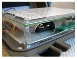
The coin battery is located right next to the power switch on the underside of the main circuit board. Be sure the main power switch is OFF before replacing the coin battery.
