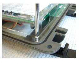
12. Reinstall the six screws that hold the circuit board holder and illuminator in the front cover of the camera case.
