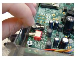
8. Insert a new 3-volt lithium battery (Panasonic BR1225 or equivalent). Be sure that the positive (+) side of the battery faces up.
