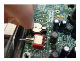
9. Slide battery into holder and be sure that the new battery is securely seated in the battery holder.
