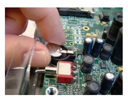
7. Remove battery by grasping between thumb and index finger.
