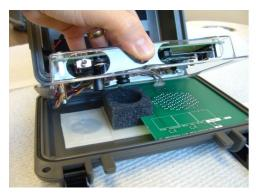
3. Carefully lift the circuit board holder off of the camera case cover.
